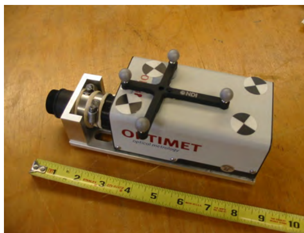
Fig. 2 Conoscope with Polaris rigid body attached
