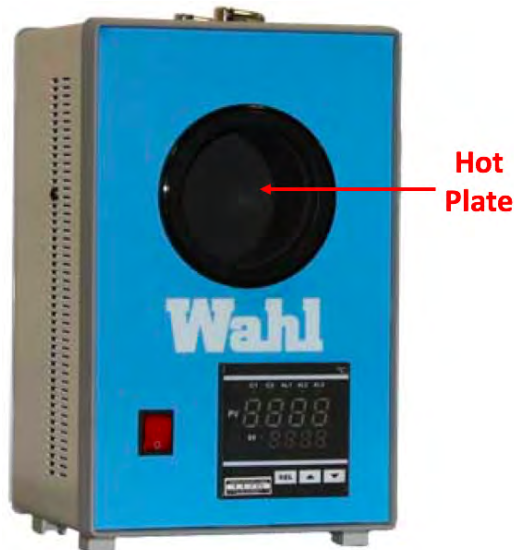
Figure 2.3: Example of hot plate type commercial blackbody (Surface Hot Plate CBB15GC, by Palmer Wahl Instrumentation Group) [27]. The temperature of the hot plate is controllable.
