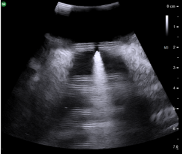
Fig. 2 Example ultrasound image of da Vinci Large Needle Driver tool tip, which provides one calibration point.
