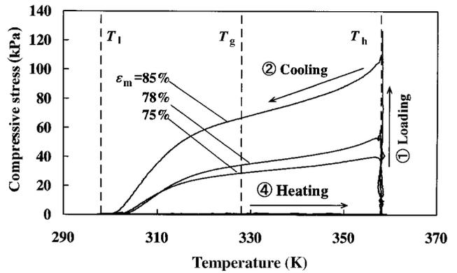
Fig. 9 Stress-temperature curves for various maximum strains
