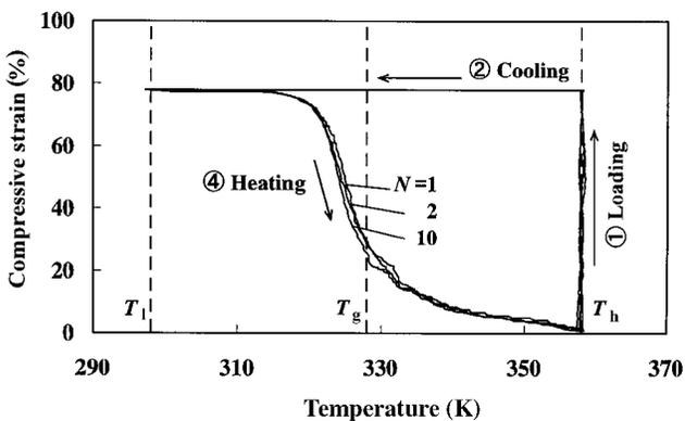
Fig. 8 Strain-temperature curves in the thermomechanical test
