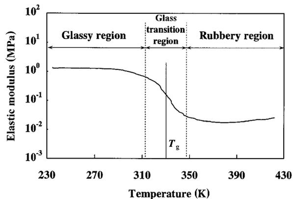
Fig. 1 Relationship between elastic modulus and temperature
