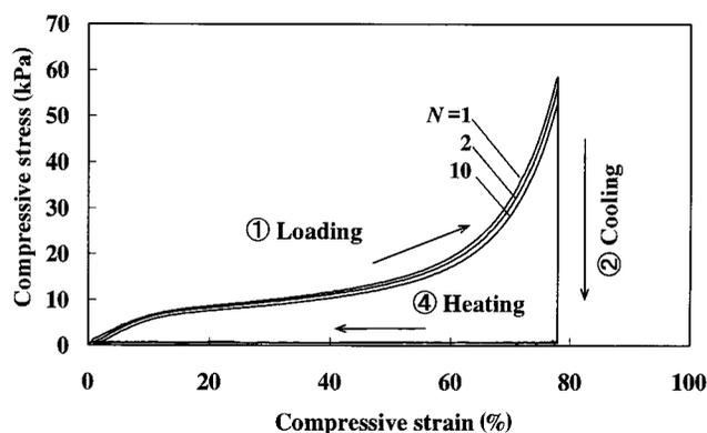
Fig. 6 Stress-strain curves in the thermomechanical test
