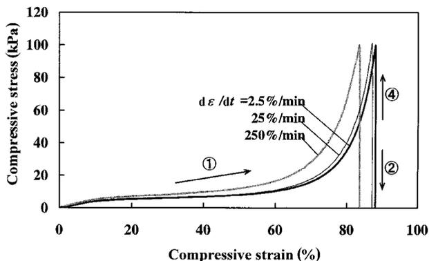
Fig. 11 Stress-strain curves in the recovery-stress test
