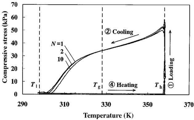
Fig. 7 Stress-temperature curves in the thermomechanical test
