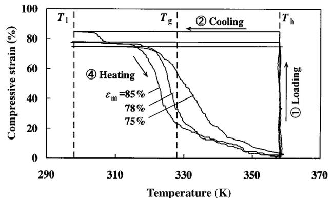
Fig. 10 Strain-temperature curves for various maximum strains
