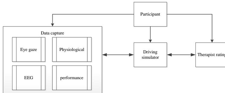
**Fig. 1.** The framework of the VR-based driving system
