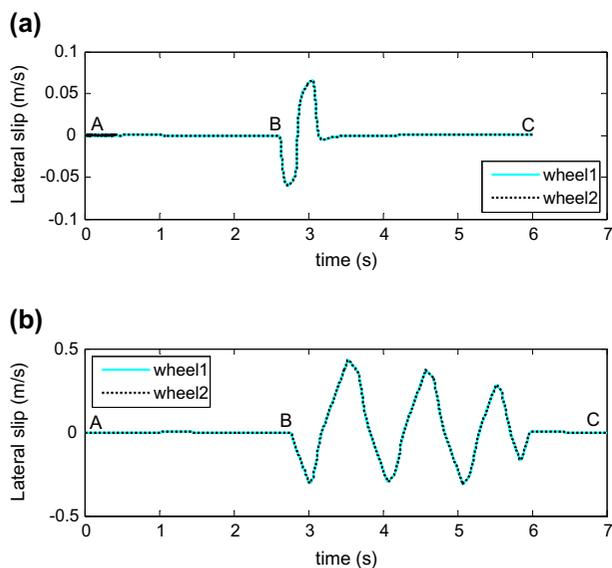
Figure 16. Lateral slip velocity on (a) Surface 1 and (b) Surface 2.
