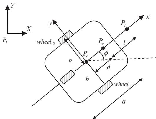
Figure 4. A two-wheeled nonholonomic mobile robot platform.
