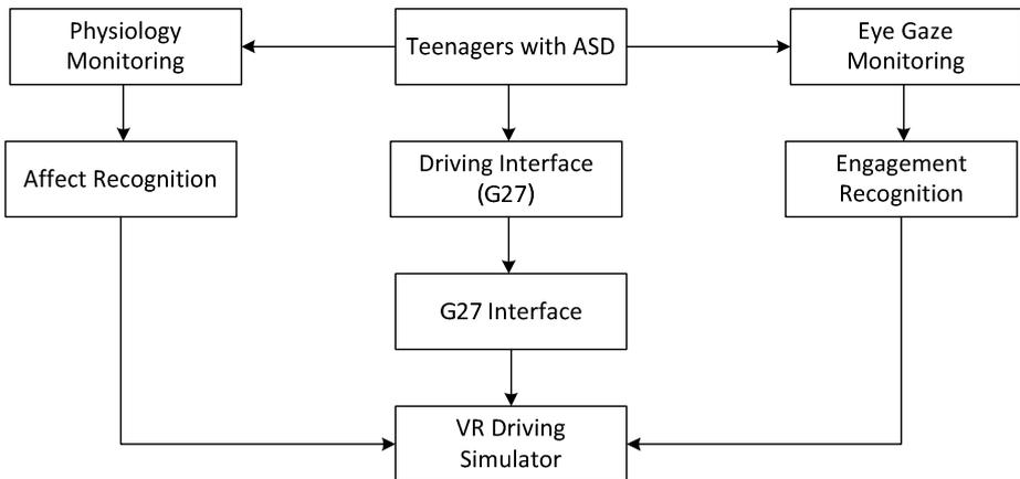
**Fig. 1.** System diagram of the adaptive driving platform
