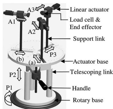
Fig. 1. Manipulation mechanism with three DoF and three DoA.
