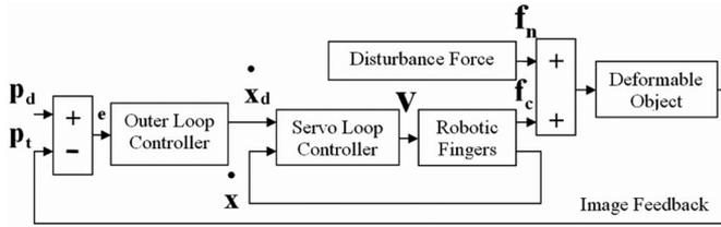
Fig. 6 Control structure for the manipulation mechanism.
