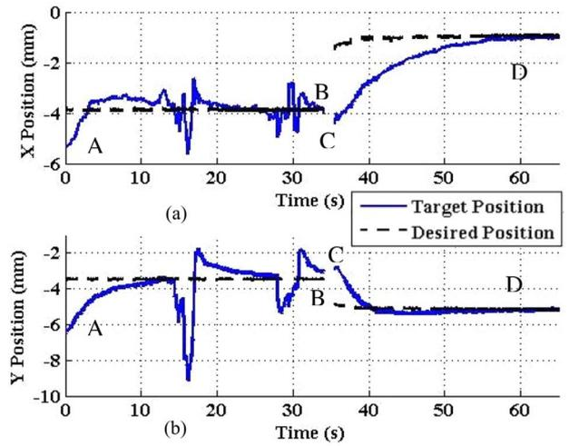
Fig. 11. Target position response with target tracking during needle insertion. (a) X displacement. (b) Y displacement.
