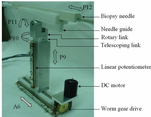
Fig. 3. Needle guidance system with four DoF and one DoA.
