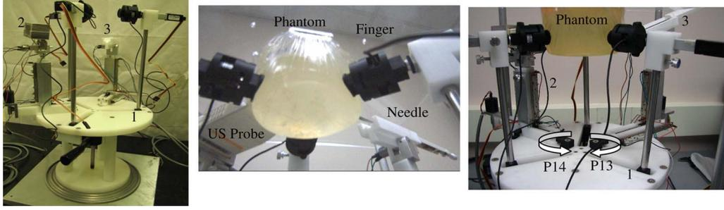
Fig. 4. Robotic image-guided breast intervention system. (a) 1—Manipulation mechanism; 2—US image acquisition system; and 3—needle guidance system. (b) (Bottom view) Phantom suspended vertically from the top. Image shows robotic fingers, US probe, and needle in contact with the phantom for a needle insertion. (c) (Side view) Image shows two additional DoF for US imaging system and needle guidance system.
