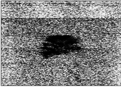
Fig. 7. US image of target in phantom. Dark blob in the image is the target.
