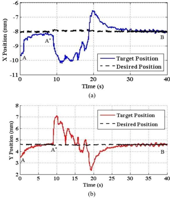
Fig. 9. Target position response during needle insertion. (a) X displacement. (b) Y displacement.
