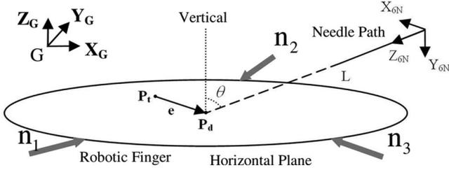
Fig. 5. Needle-target alignment during breast intervention. The horizontal plane passing through the target represents a cross section of the breast.
