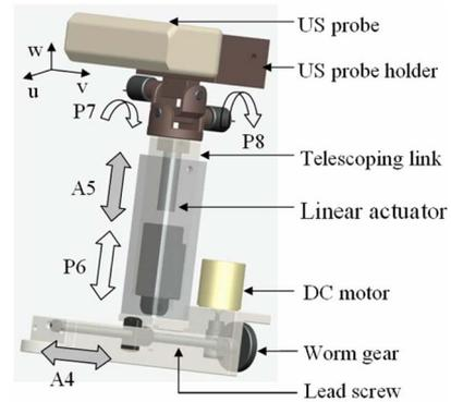
Fig. 2. Autonomous US image acquisition device with three DoF and two DoA.
