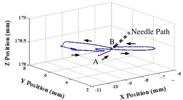
Fig. 8. Target and nominal needle paths during needle insertion.
