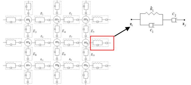
Fig. 2: Model of a rheological object with interconnected mass-spring-damper.  $k_1$  is the spring stiffness,  $c_1$  and  $c_2$  are the damping coefficient of non-residual and residual deformation part, respectively.
