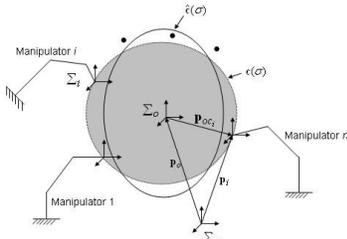
Fig. 1: Schematic of manipulators handling a deformable object.
