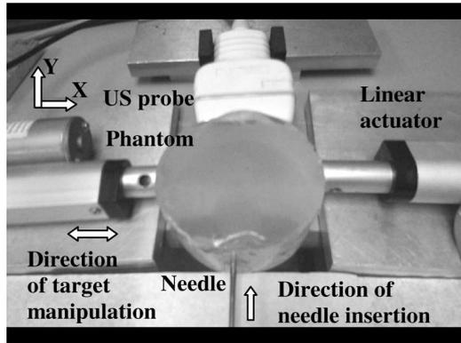
Fig. 13. US experimental setup. Needle is inserted along Y-axis and actuators control target position along X-axis.
