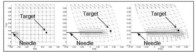
Fig. 1. Finite-element model of needle insertion in soft tissue [3]. (a) Cross section of 3-D model shows the finite-element mesh. (b) Target movement during needle insertion.
