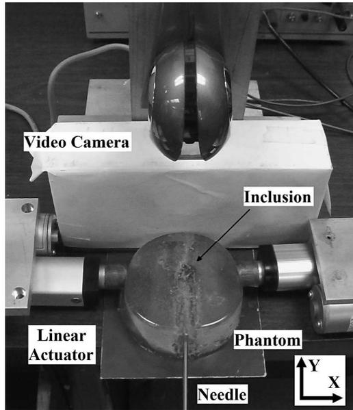
Fig. 10. Experimental setup for needle insertion task. Needle is inserted along Y-axis. Actuators control target position along X-axis.
