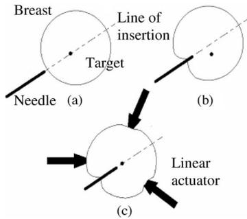
Fig. 2. Needle insertion schematic. (a) and (b) Target movement during needle insertion. (c) Minimizing needle–target misalignment using external actuators.
