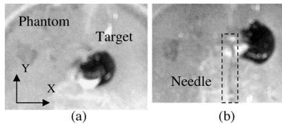
Fig. 6. Images grabbed from the video signal during needle insertion in inhomogeneous phantom. (a) Initial position of target in phantom. (b) Displacement of target from needle path. Needle is identified in the figure with a dotted bounding box.
