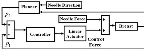
Fig. 4. Control structure for planar target position control.
