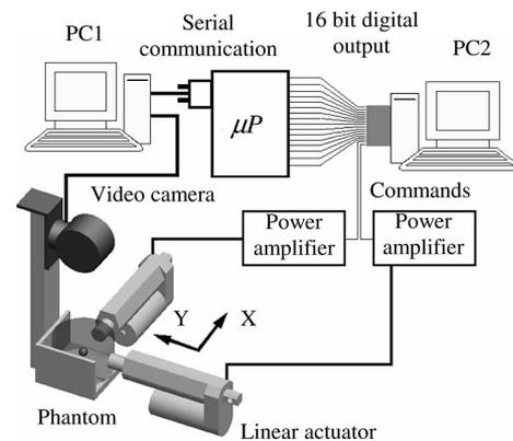
Fig. 8. Experimental setup shows system architecture and the location of actuators for target position control.
