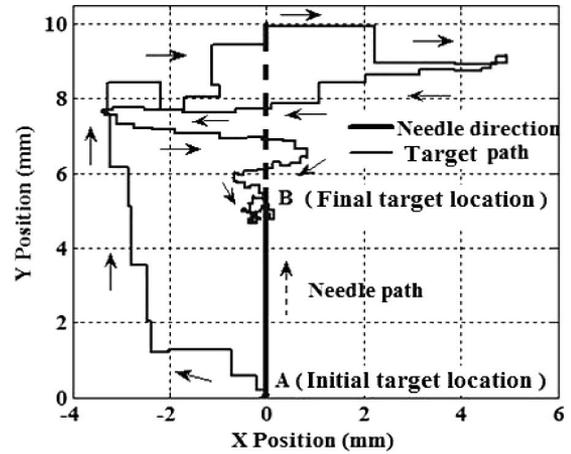
Fig. 12. Locus of target position for trial 1. Needle is inserted along the Y-axis. Point A is the initial target location and point B is the final target location.
