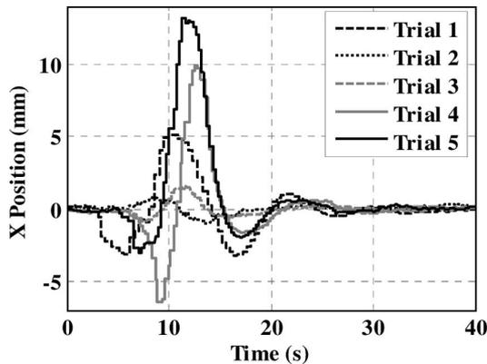
Fig. 11. Target position response during needle insertion. Plot shows that the target reaches the needle path in approximately 28 s.
