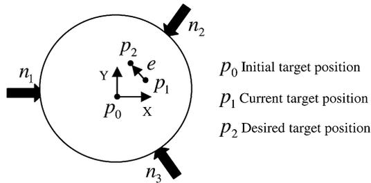
Fig. 3. Schematic of actuator and target geometry. Three external actuators are used for planar target position control.
