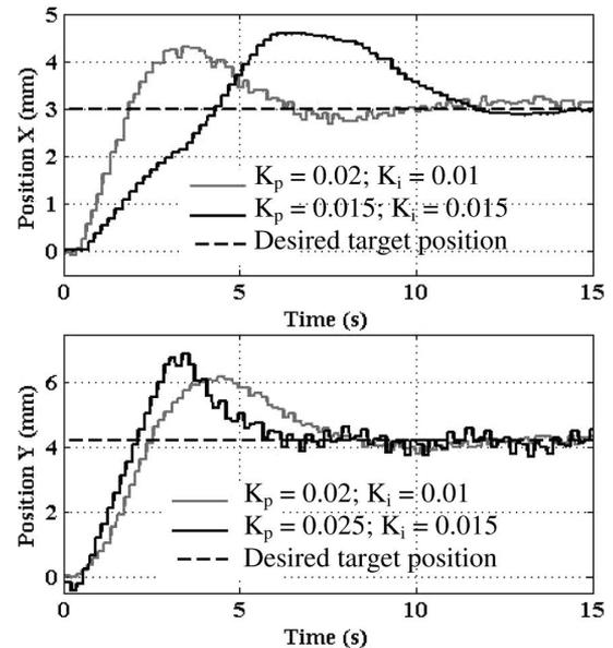
Fig. 9. Target positioning in horizontal plane. Position response of the target for two trials with different control gains. Target reaches the desired position in approximately 12 s with  $K_p = 0.02$  and  $K_i = 0.01$ .
