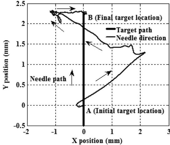
Fig. 15. Locus of target position for *experiment 4*. Needle is inserted along the Y-axis. Point A is the initial target location and point B is the final target location.
