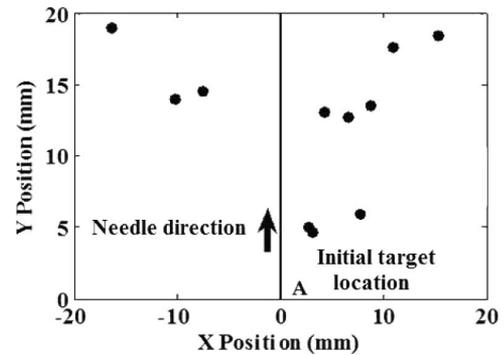
Fig. 7. Movement of target during needle insertion. Needle is inserted along  $Y$ -axis. Dots indicate maximum displacement of target from the needle path.
