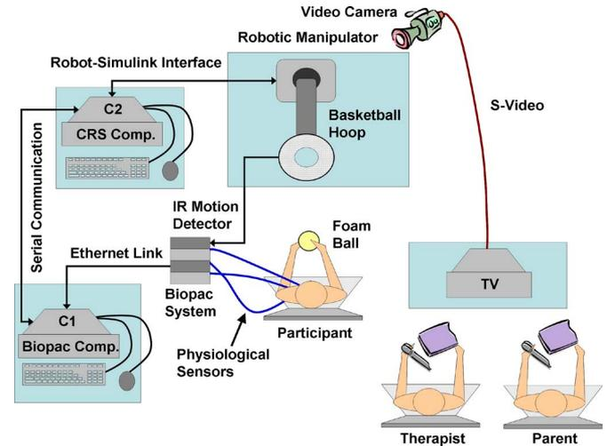
Fig. 5. Experimental setup for robot basketball.
