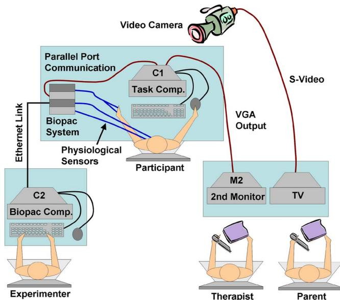
Fig. 2. Experimental setup for affective modeling tasks.
