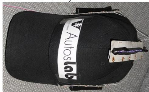
Fig. 5 The hat holds the array of LEDs at side and top.
