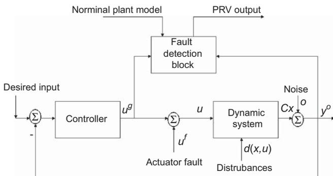
Fig. 1. Schematic diagram of the FDI system.
