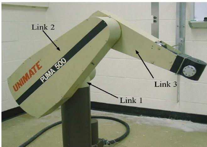
Fig. 2. Unimate PUMA 560 robot manipulator.
