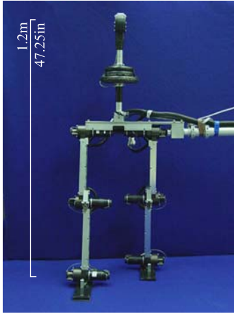
Fig. 4. Experimental prototype of a 7-link dynamic walker developed at the Vanderbilt University - Center for Intelligent Mechatronics
