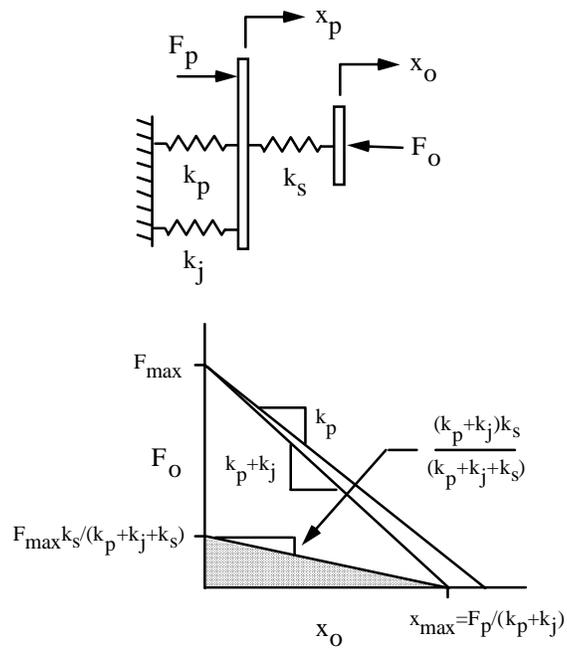
Figure 13. (TOP) Quasi-static model of PZT with compliant mechanism joint stiffness and structural compliance and (BOTTOM) region of attainable output (region of operation).
