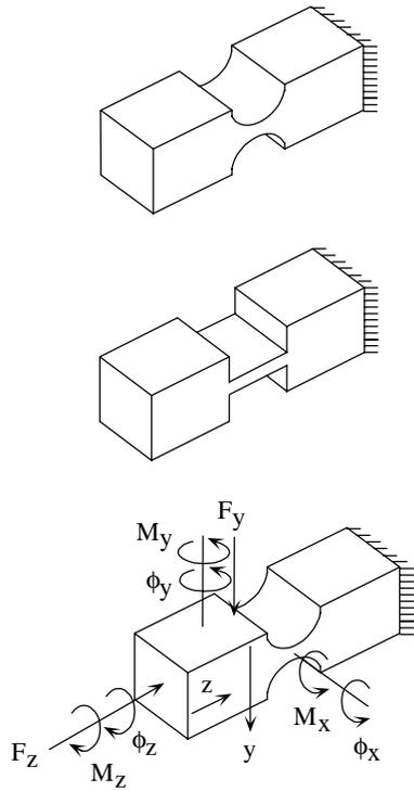
Figure 10. (TOP) Typical flexure geometry, (MIDDLE) thin, flat flexure geometry, such as the super-elastic flexure of Horie et al., and (BOTTOM) loading diagram illustrating the stiffness along the direction of rotation and compliance in all other directions.
