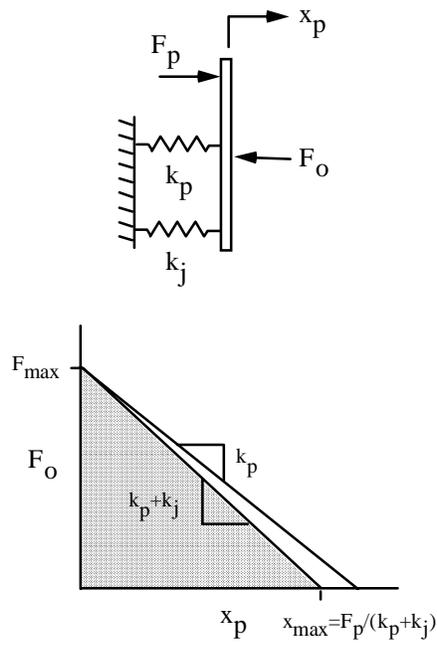
Figure 12. (TOP) Quasi-static model of PZT with compliant mechanism joint stiffness and (BOTTOM) region of attainable output (region of operation).
