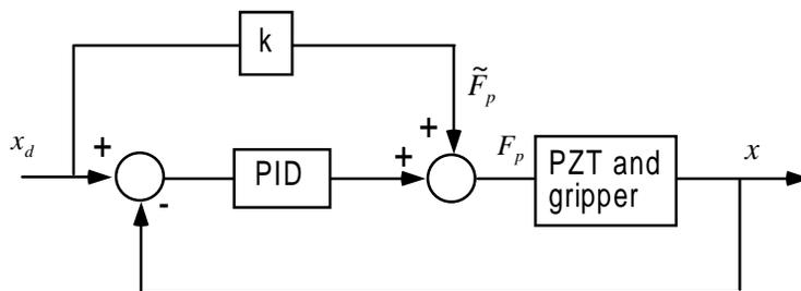
Figure 4. PZT-actuated compliant mechanism position controller. The feed-forward term is a simple quasi-static model of the PZT and compliant mechanism (i.e., a pure stiffness), which provides a command estimate for the desired position, and the PID loop provides correction of the estimate for model error.
