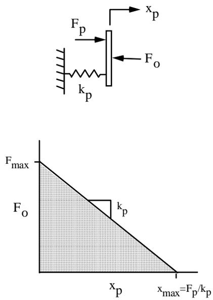
Figure 11. (TOP) Quasi-static model of PZT stack actuator and (BOTTOM) region of attainable output (region of operation).
