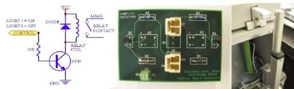
Figure 4. Electronic interface board and lid.
