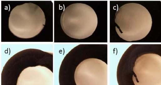
**Figure 8.** (a), (b) Cross-section views of capillary cut at 0.8W and 30rpm; (c), (d): 0.8W and 40rpm and (e), (f): 0.8W and 50rpm.
