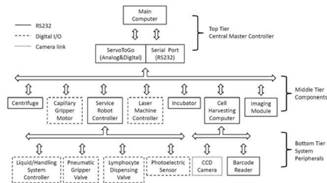
Figure 3. Hardware architecture.
