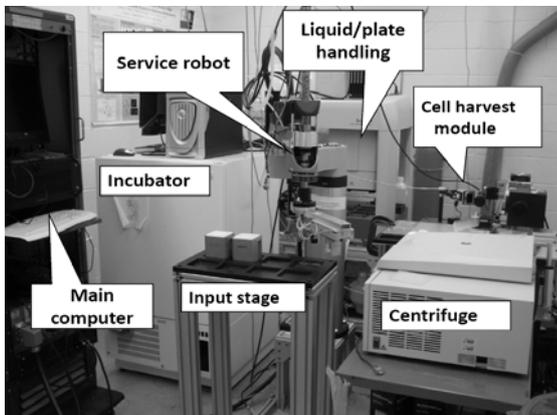
Figure 1. System breadboard prototype.
