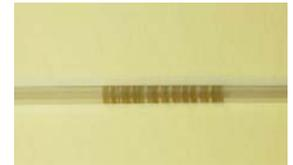
**Figure 7.** Barcode on the capillary.
