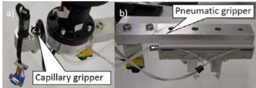
**Figure 5.** Multi-purpose material handling gripper.
