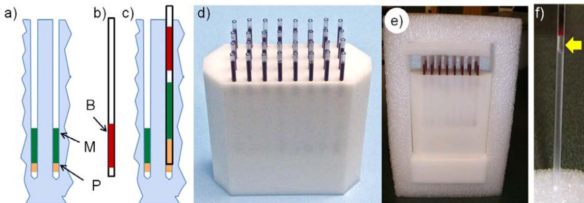
Figure 3: Scheme of the sample collection. a) sample holder with sealing putty (P) and separation medium (M), b) Blood in a capillary (B), c) capillary loaded into sample holder layering blood above the separation medium without mixing. d) Photo of filled capillary holder. e) Samples packaged for shipping. f) Blood-filled capillary removed from holder after shipping from ASU. Note that the air gap between the separation medium and blood is intact.
