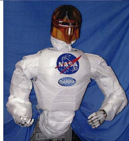
Robotic car assembly plant of Ford Motor Company at Michigan as an industry example (Top), NASA Robonaut dual-arm humanoid torso for space applications as a research example (Bottom).
