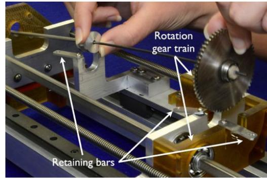
Fig. 6: Quick-release mechanism for the tubes. Either tube may be quickly released from the mechanism by removing a screw and swinging a retaining bar out of the way. This enables one to change the inner tube during a surgery if multiple tubes with different curvatures are to be used in sequence.
