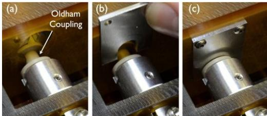
Fig. 5: An Oldham coupling is used to transfer rotation of the motor shaft through a tortuous path to the sterile lead screws and square shaft for translation and rotation of the cannula tubes. (a) Oldham coupling made from PEEK plastic. (b) An aluminum plate is brought down over the Oldham coupling and secured in place. (c) The aluminum plate creates the tortuous path between the non-sterile bagged motor pack and the sterile robot.
