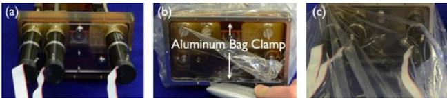
Fig. 4: The motor pack is bagged to ensure sterility of the robot for clinical use. (a) The motor plate, shown here, is removed from the robot to allow the bag to be attached with the aluminum bag clamp. (b) After the bag clamp is attached, the portion of the bag inside the bag clamp is removed, enabling the motors to subsequently attach to the Oldham couplings. (c) The motor plate is reattached and the bag pulled over it. The robot is now sterile.
