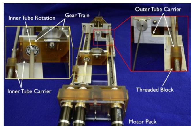
Fig. 2: The robot uses lead screws to translate the carriers via a threaded block. The carriers, which hold the tubes, travel along a linear track. The inner, precurved tube is rotated with a square shaft attached to a small gear that meshes with the large gear attached to the tube hub.
