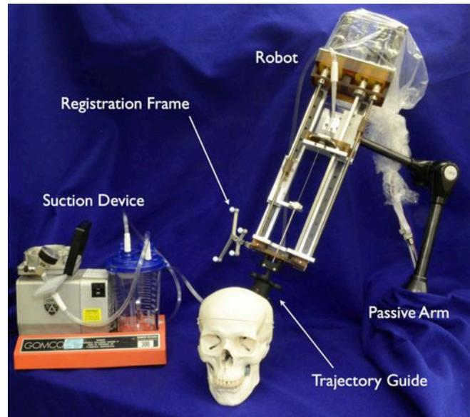
Fig. 1: The complete system is shown attached to a phantom skull with the trajectory guide. The robot is supported with a passive arm, and a suction device is attached to the robot to aspirate the hematoma. The motor pack attached to the robot is bagged for sterility, while the rest of the robot is autoclavable. The optical tracker used for image guidance is not shown, although the rigid body it tracks can be seen attached to the robot.
