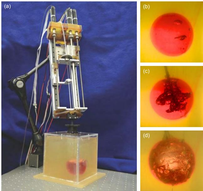
Fig. 10: Phantom experiment. (a) The robot is attached to the passive arm and secured to the trajectory guide which is mounted onto the top of a acrylic box. The active cannula is deployed to the clot and the aspiration tube is used to debulk the clot. (b) The blood clot is shown prior to beginning the experiment, (c) progress midway through the removal experiment, and (d) the same area after aspiration.
