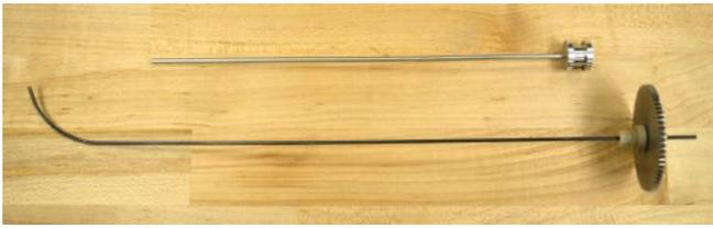
Fig. 3: The tubes are permanently attached to hubs using a biocompatible glue and can be autoclaved. The inner, precurved tube also has a gear attached to the hub to rotate the tube.
