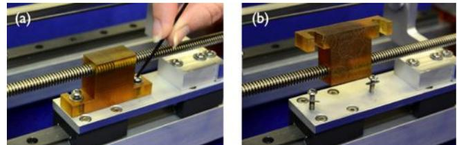
Fig. 7: Quick-release mechanism for carriers enabling them to be detached from the lead screws and manually slid backward, for manual rapid tube retraction. The mechanism works by (a) loosening holding screws, followed by (b) swinging the threaded block away from the carrier.
