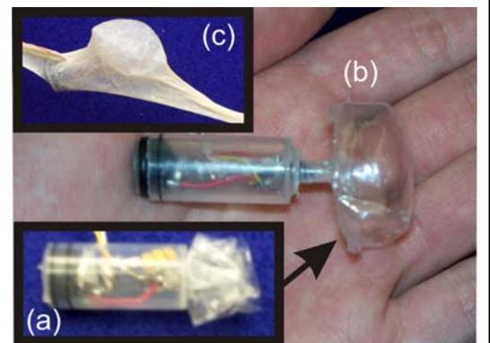
**Figure 3.** Proof of concept capsule showing (a) initial deflated state (b) balloon inflation when valve activates, and (c) inflation within ex vivo porcine intestine.
