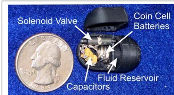
**Figure 2.** Internal components of the insufflation system: two 3V batteries charge 3 capacitors that fire the solenoid valve. In our initial proof-of-concept study we have packaged all components in a 26 mm long by 11 mm diameter capsule.
