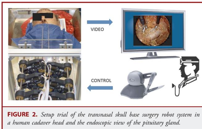
**FIGURE 2.** Setup trial of the transnasal skull base surgery robot system in a human cadaver head and the endoscopic view of the pituitary gland.
