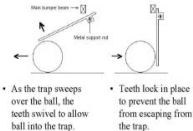
**Figure 6: Ball trap mechanism.**
