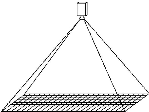
**Figure 1: An overhead fixed camera causes pixels to correspond to physical Cartesian coordinates**
