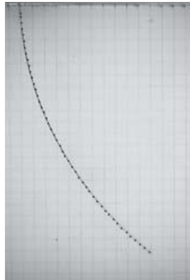
Fig. 7. Tip positions during needle insertion shown overlaid on the final needle path. Tip positions were extracted automatically from insertion images.
