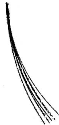
Fig. 13. The final needle locations, extracted from difference images, with different bevel angles illustrate the steering effect of the bevel tip. A 5^\circ bevel exhibits the most bending while an 80^\circ bevel the least.
