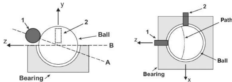
Fig. 4. The positions of the drive wheels (1 and 2) result in additional frictional contact and off-axis ball rotation (axis B is desired and axis A is the result). The path of a point under the user's fingertip is then curved as shown.
