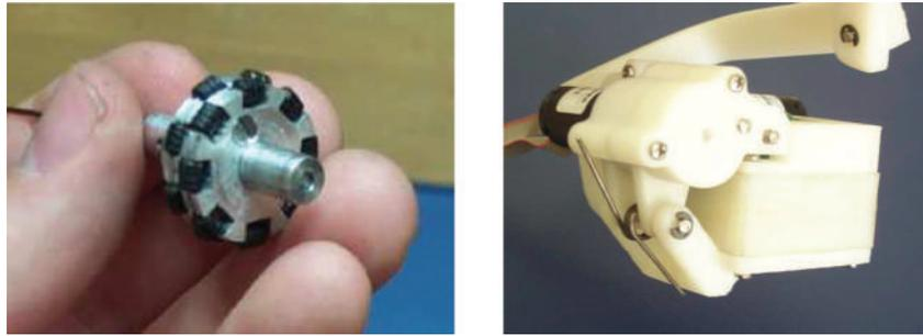
Fig. 3. (Left) The omniwheel from Murphy et al. [2004]. (Right) The drive wheel modules are spring-loaded against the ball.
