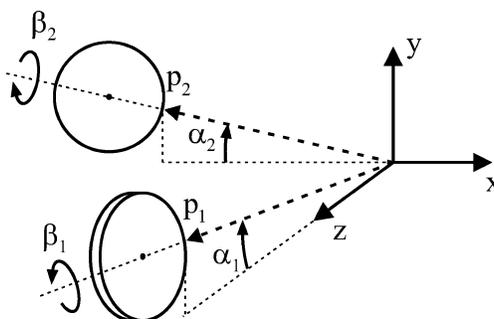
Fig. 6. Angle and vector definitions for the slip display. The two drive wheels are shown, while the ball (omitted from the figure) is centered at the origin.
