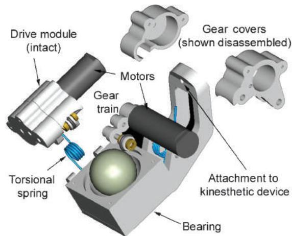
Fig. 2. An exploded view of the device assembly shows the various parts of the tactile slip display.
