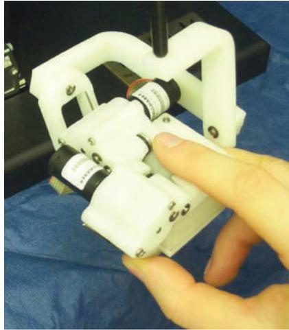
Fig. 1. The two-degree-of-freedom slip display mounted on the output link of a PHANTOM haptic device.
