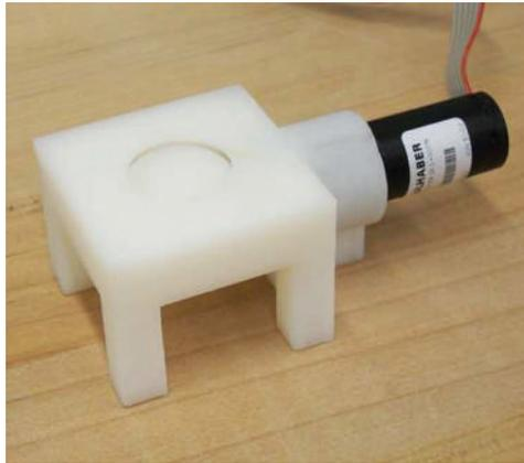
Fig. 7. Single-axis slip device used in psychophysical experiments consisting of a 25.4 mm ball attached to the drive shaft of a motor. The user interacts with the ball in the same manner as in the 2 DOF slip display.
