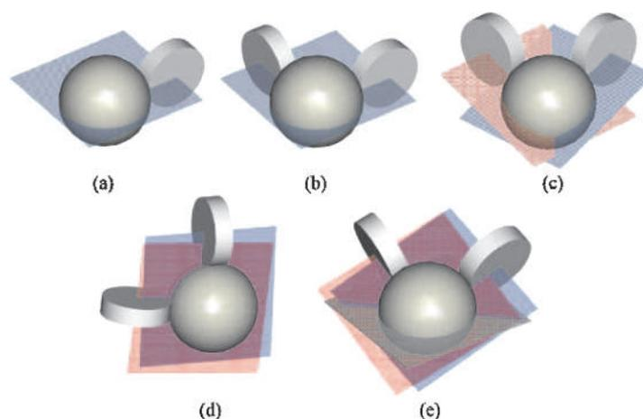
Fig. 5. (a) Considering one wheel only, the axis of rotation of the ball can be anywhere in the plane shown. (b) Wheels on equator share a common plane of permissible axes. (c) Wheels off the equator constrain rotation axis to a line. (d, e) Tilting the drive wheels properly regains 2 DOF motion by realigning constraint planes.
