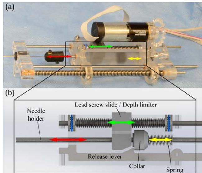
**Fig. 5.** (a) View of the piercing mechanism used to impart a rapid motion to the piercing needle that creates a needle-sized port in the bronchial wall. (b) In the piercing mechanism, the lead screw slide compresses a spring until the collar is secured by the release lever. Upon triggering the release lever, the needle holder is propelled forward until it contacts the lead screw slide, controlling the depth of the piercing needle.
