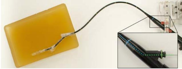
**Fig. 7.** The experimental setup used for the system feasibility and accuracy experiments as described in Sec. 5.1 consisted of a phantom bronchial tree (made from plastic tubes) that was embedded in phantom parenchyma (gelatin). The inset shows the bronchoscope handle and the sharp bend in the working channel, which is discussed further in Sec. 6.
