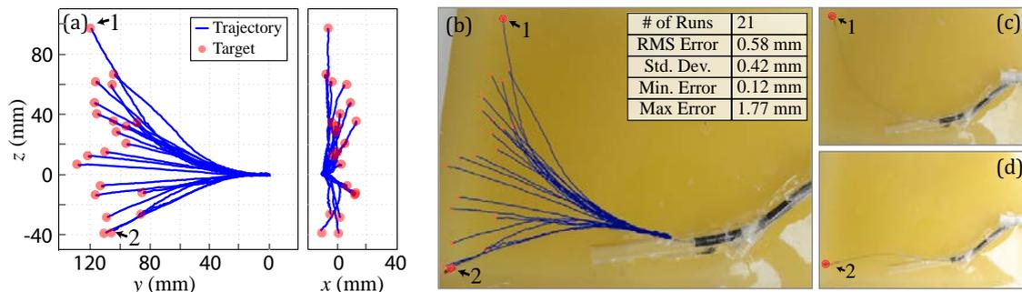
**Fig. 8.** (a) Phantom targeting experimental results of 21 insertions as described in Sec. 5.1. (b) The 21 targeting trials are overlaid on the experimental setup. Trials 1 and 2 are explicitly shown in (c) and (d).
