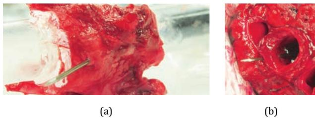
**Fig. 9.** (a) *Ex vivo* porcine bronchial tissue was wrapped around a PVC tube representing a bronchial tube. The piercing mechanism was used to fire the piercing needle through the tissue, as shown here. This creates a port in the bronchial wall for the concentric tube robot and steerable needle to deploy through. (b) The piercing mechanism was also tested in whole samples of porcine lung, shown here.
