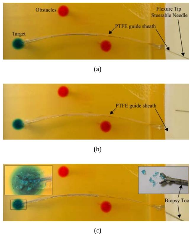
**Fig. 12.** A preliminary investigation into the use of a guide sheath for biopsy is shown. (a) First, a PTFE guide sheath was passed over a flexure-tip steerable needle that had reached the target, (b) the needle was removed through the sheath, creating a path to the target, (c) then a flexible biopsy tool was inserted through the guide sheath and used to obtain core samples of the gelatin target.
