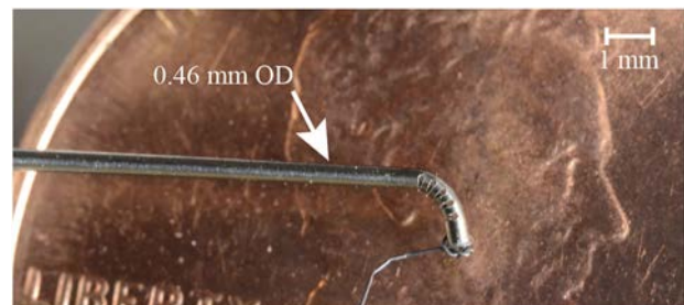
Fig. 13 A 0.46 mm OD wrist was made using wire EDM manufacturing and is shown being deflected to approximately 90 deg. It is overlaid here on a penny to provide a sense of scale. For this photograph, the tendon was tied at the end of the wrist since the end caps made for the 1.16 mm wrist prototype were much larger than the 0.46 mm tube.
