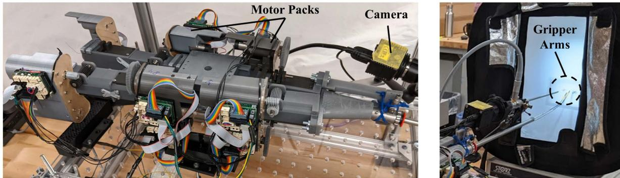
Figure 4. Left: Proposed two-manipulator disposable concentric tube robot with modular motor and electronic packs (10 DoF). Right: View of experimental setup for ring transfer task
