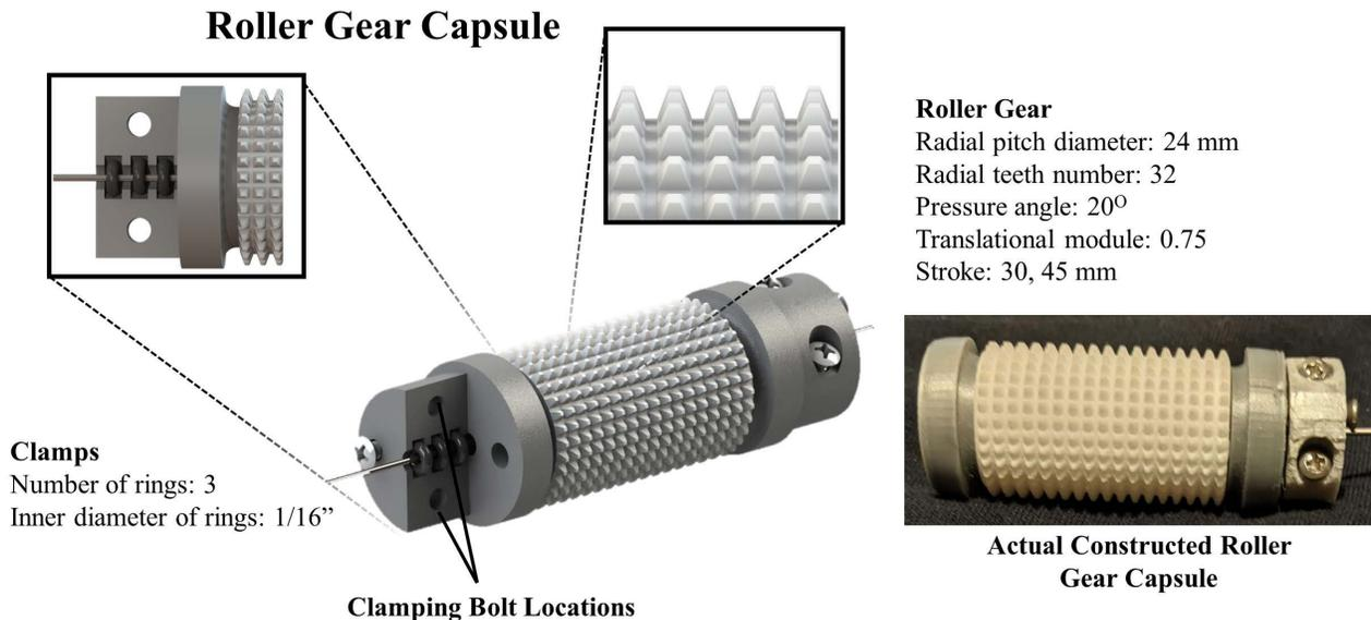
Figure 2. Roller gear capsule along with o-ring clamps for tube grasping.
