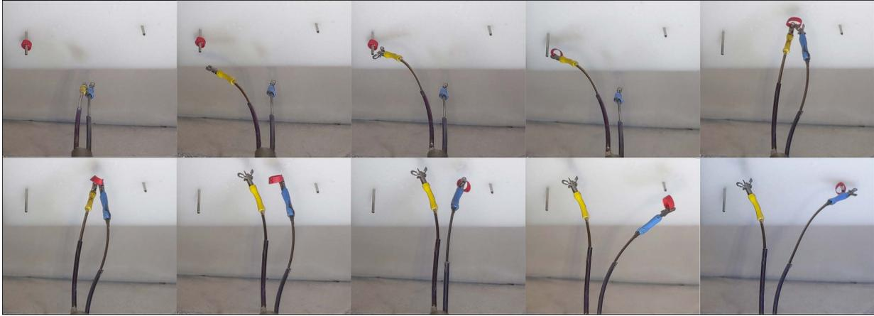
Figure 5. Ring transfer results. From left to right and top to bottom: the initial robot state, left manipulator actuation to target, transfer process to right manipulator, and right manipulator actuation and placement of the ring onto second target are shown.
