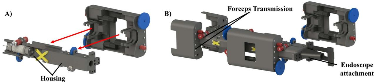
Figure 3. a) Two module sets CTR configuration used in repeatability experiment. b) Six module sets CTR configuration used in bimanual cooperation experiment.
