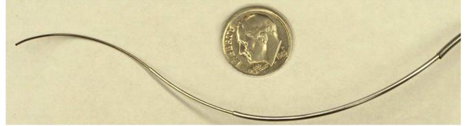
Fig. 1. Prototype active cannula made of three superelastic nitinol tubes and one central wire.
