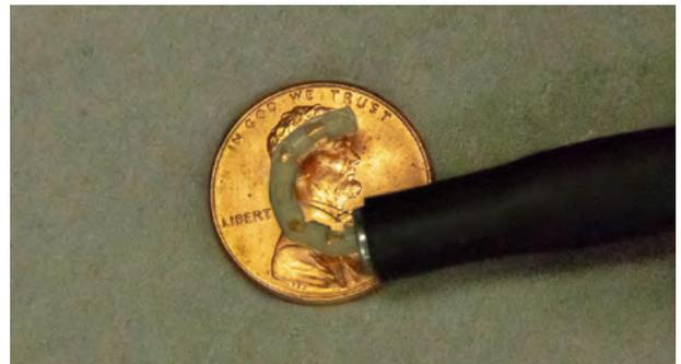
**Figure 2:** Prototype luminal manipulator delivered through a 6 mm diameter bronchoscope.
