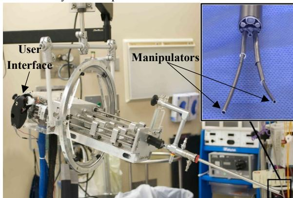
Figure 1: The hand-held robot from [3] delivers two concentric tube robot manipulators. These manipulators are controlled by a user interface which is mounted to the system.
