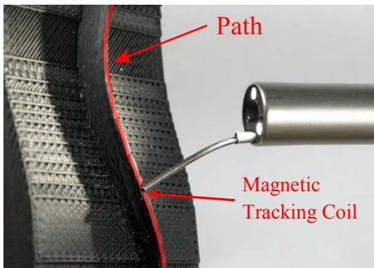
Figure 3: The path following experimental setup. During this experiment, the user commanded the tip of the manipulator to follow the path as accurately as possible.
