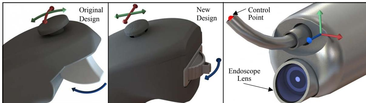
Figure 2: (Left) The original user interface design features a pivoting joystick and a unidirectional trigger. (Middle) The new design features a sliding joystick and a bidirectional dial. (Right) The control point is located at the tip of the concentric tube manipulator. The colors of the arrows in each user interface image indicate the directional velocity that is commanded to the control point in the coordinate system fixed to the tip of the endoscope.
