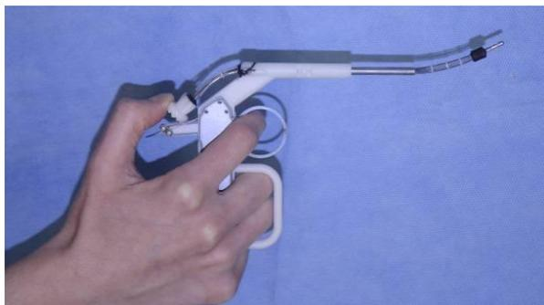
Figure 4: Prototype deflecting upward under hand control.
