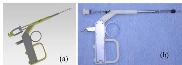
Figure 2: (a) CAD model of tool design, (b) prototype of tool
