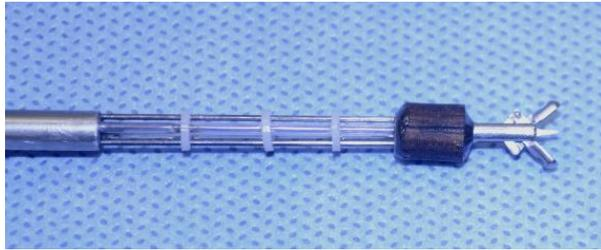
Figure 3: Multi-backbone bending mechanism with grasper
