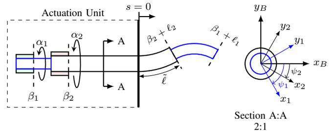
Fig. 1: Model parameters, kinematic variables, and coordinate frames for the concentric tube model.
