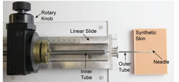
Fig. 5: The top view of the experimental setup.
