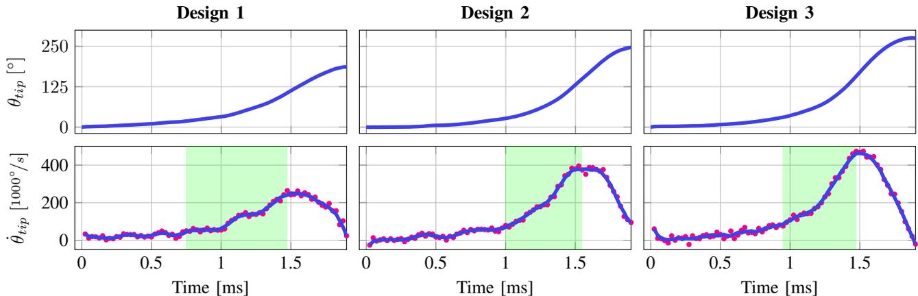
Fig. 8: The angular position and velocity of the tip of the manipulator. A moving average of the angular position is plotted and the raw angular velocity data is overlaid with a moving average. The shaded region  $\square$  indicates the duration of snap, with limits defined by the time when the needle has reached 20% of its maximum velocity and when the needle has reached its maximum velocity.
