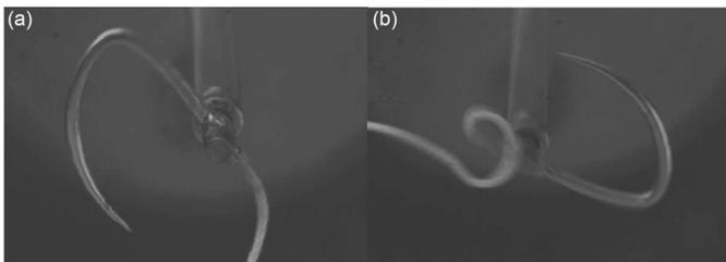
Fig. 4: (a) The moment just before the elastic instability. (b) The moment after the instability for Design 2.
