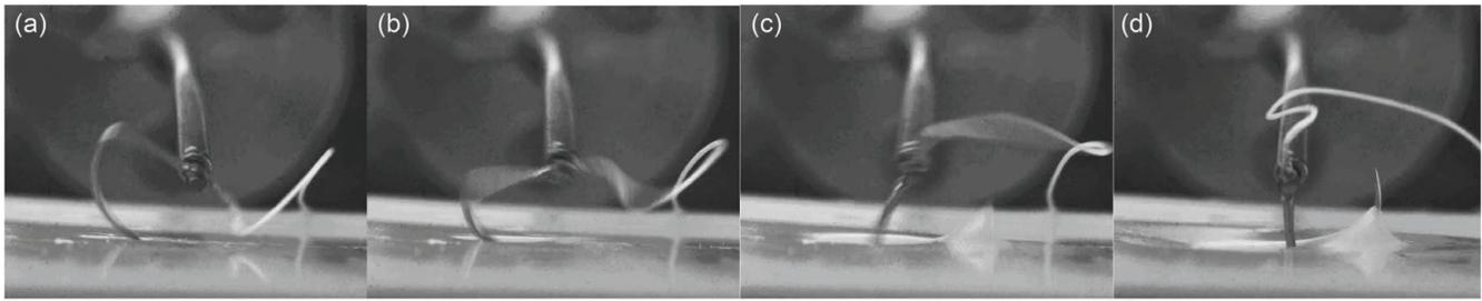
Fig. 6: A series of frames taken with the high-speed camera as the concentric tube manipulator moves through an elastic instability. These are images from the elastic instability of the configuration with the highest predicted energy release.
