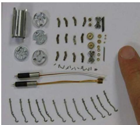
**Figure 3.** Fabricated internal mechanical components of the capsule robot before assembly. The assembly procedure is discussed in section 5, and the assembled prototype is shown in figure 1.
