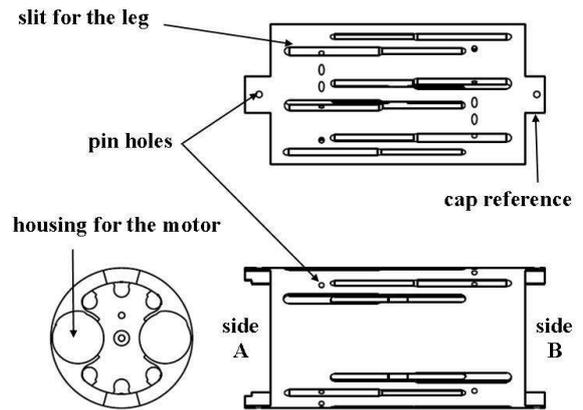
**Figure 6.** The capsule body is 11.1 mm in diameter, 23.6 mm long and its smallest features are 12 holes of 0.4 mm diameter.
