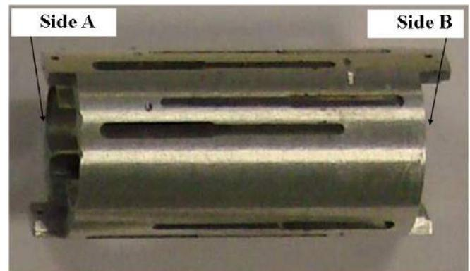
**Figure 7.** The fabricated capsule body, made from Ergal.
