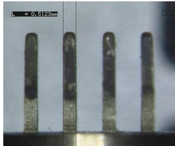
**Figure 14.** A photo taken after using the electrode negatives to create the leg seat pockets in the leg holders. This photo shows four electrodes 0.9 mm wide by 0.5 mm thick after a single use.
