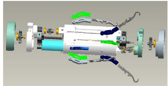
Figure 24. Exploded view of the capsule robot.
