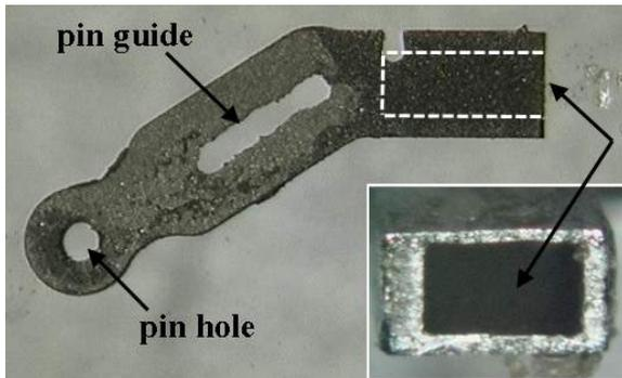
**Figure 13.** A longitudinal section of the leg holder. Its total length is 7.38 mm, while its minimum feature, the pin guide, is 0.4 mm wide. The inset shows the leg seats.
