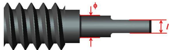
**Figure 15.** Drawing of the lead screw tip that interfaces with the gear.  $\phi = 0.45$  mm and  $l = 0.28$  mm.
