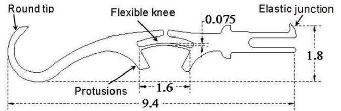
**Figure 10.** An example schematic drawing of a capsule robot leg. All dimensions are in mm.
