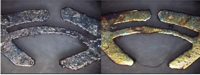
Figure 19. Two leg flexure joints machined with different techniques: (left) wire EDM; (right) laser cutting.
