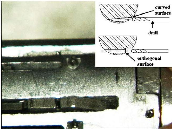
**Figure 9.** The levelled surface for the hole. Inserted into the hole is a pin within a bushing. The inset line drawing shows the trajectory of a drill bit on rounded versus levelled surfaces.
