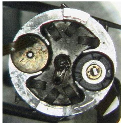
**Figure 8.** An axial view of the capsule, showing assembled motors (right and left circular parts) and the central nut.
