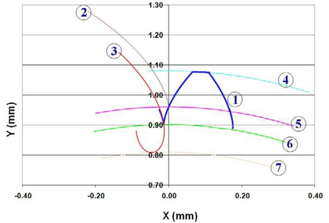
**Figure 17.** Shown above are curves taken from the output of the spreadsheet software that were used to define the gear tooth shape: (1) tooth profile, (2) evolute curve; (3) profile of the curve easing; (4) addendum circle; (5) pitch circle; (6) base circle; (7) root circle.
