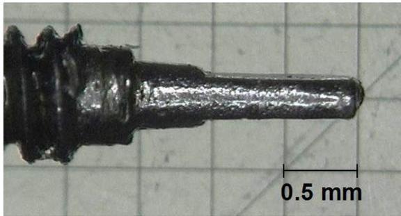
Figure 22. Optical microscope image of the lead screw tip.
