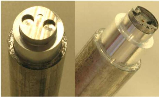
**Figure 5.** The custom cap fixture used for refixturing the caps on the machine. The holes shown are 3.95 mm in diameter. The right image shows the fixture with a cap in place on it, just after machining the cap's second face.
