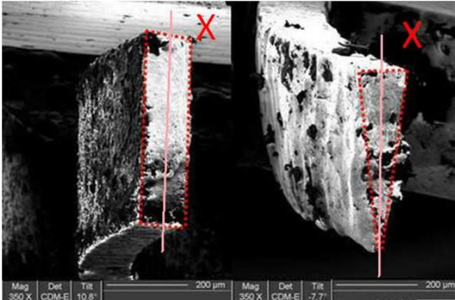
Figure 20. Cross-sections of knee flexure joints manufactured, using (left) wire EDM, and (right) laser cutting.
