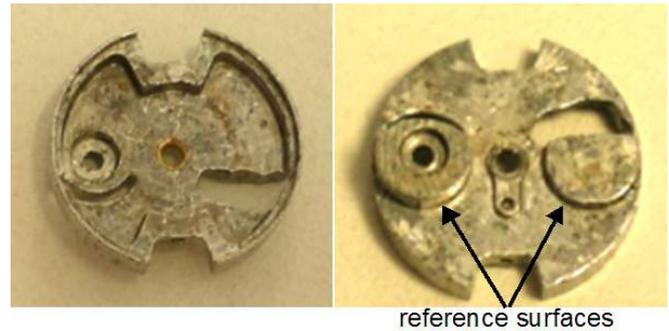
**Figure 4.** The two faces of one of the caps. The two cylindrical protrusions, that are the reference surfaces, are 3.85 mm in diameter and the inter-axis spacing is 6.8 mm.
