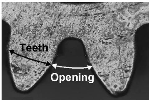
Figure 23. Picture of the tooth profile taken by the VideoCheck machine.
