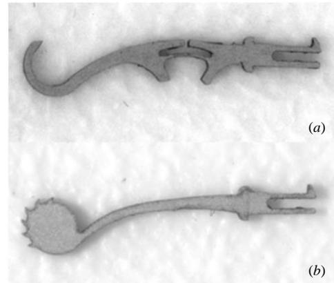
**Figure 11.** Two example of leg designs for the capsule robot.
