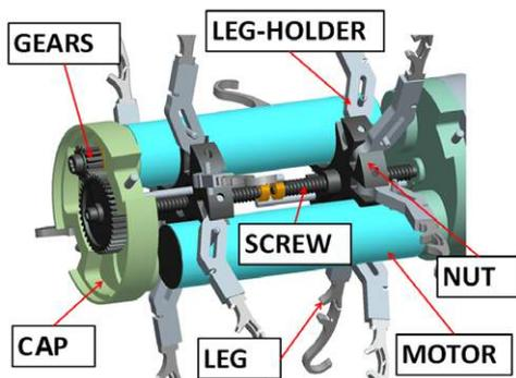
**Figure 2.** CAD drawing of the assembled internal components of the capsule robot. Component dimensions range from 23.6 mm (length of the capsule body) to 0.4 mm (diameter of the pins).
