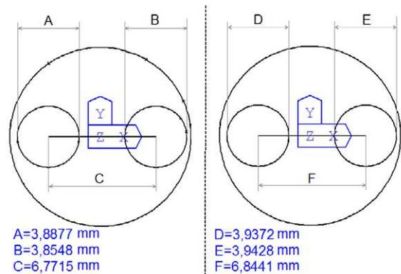
**Figure 18.** Measurement data from the VideoCheck machine. The cap (left) and the cap fixture (right).
