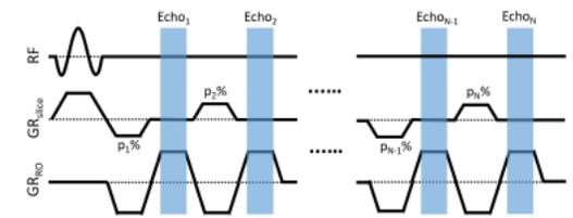
Figure 1: Pulse sequence diagram for the multiple-echo Z-shimmed sequence. Each echo was shimmed separately in the slice dimension by a percentage,  $p$ , of the full refocusing gradient area. For this application, gradient areas were allowed to vary between 0% and 200% of the full refocusing gradient area.
