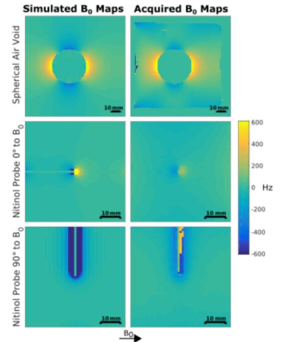
Figure 2: (Left) Field maps simulated using the developed tool for a spherical air void (40 mm  $\Phi$ ) and a nitinol ablation probe (1 mm  $\Phi$ ) at two orientations within the magnetic field. (Right) Acquired field maps of the objects in a 3T scanner ( $\Delta TE = 1$  ms, Philips Achieva). High order field variations
