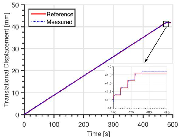
Fig. 3 Translational displacement tracking
