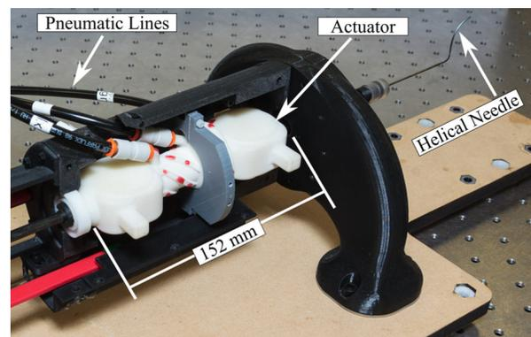
Fig. 1 Robot with helical steerable needle
