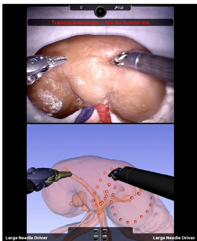
Kinematics-based tool tracking.
