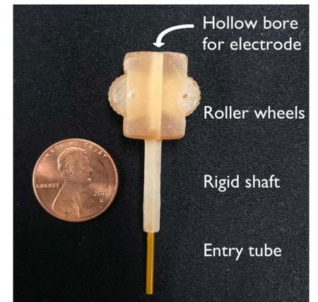
**Figure 2.** Electrode insertion tool ensured that electrodes were inserted in a linear vector matching the intended trajectory. Electrodes were placed in center of tool and opposing wheels were rolled by hand to push electrodes through shaft.
