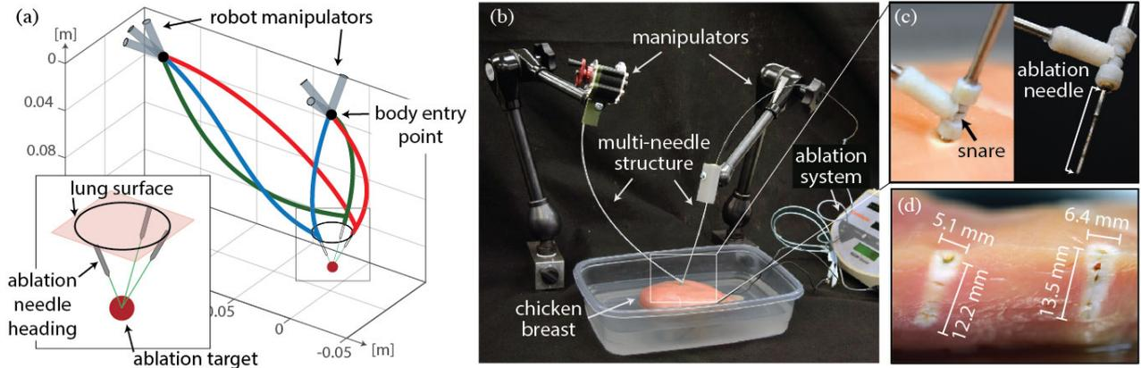
**Fig. 3:** (a) Simulation experiments demonstrate aiming dexterity by illustrating how the tip of the prototype multi-needle system can be maneuvered along a circular trajectory on a simulated lung surface while keeping it aimed at a subsurface lung nodule. (b) The prototype multi-needle structure is sufficiently stiff to insert an ablation needle (c) into chicken breast for ablation tasks (d).
