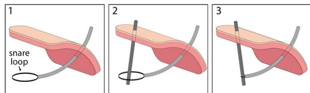
**Fig. 2:** A multi-needle structure is assembled inside a body cavity using snares that form structural grasps when tightened. The assembly of a two-needle structure is shown in three steps.
