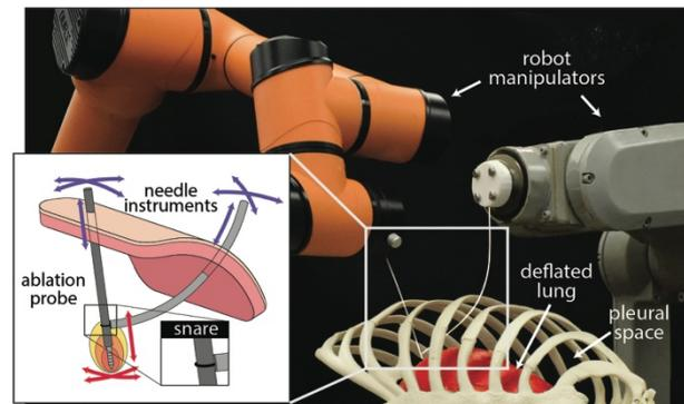
**Fig. 1:** A multi-needle system is assembled inside a body cavity and is maneuvered by manipulating the needles outside the body using robot manipulators. The needles bend each other to produce coordinated motion inside the body.
