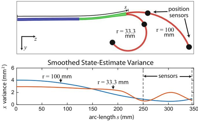
**Fig. 3** The effect of changing a concentric-tube robot’s inner-tube curvature on the smoothed state-estimate position variance in the  $x$  direction (out of the page) is shown (the variance in the  $y$  and  $z$  are largely unchanged). The smoothed estimate is found using the methods in Sect. 3.1 with two backbone-position sensors arranged on the robot as depicted. The covariances used by the smoothed estimator are for the physical robot reported in Sect. 3.2
