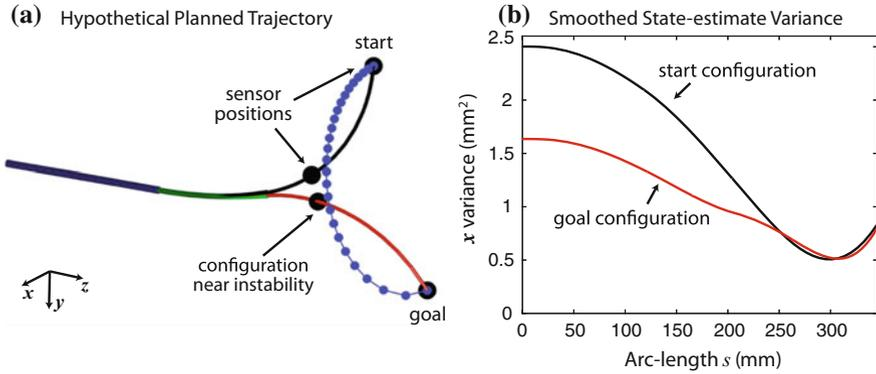
**Fig. 5** The effect of changing the input  $u(x_0)$  to follow a hypothetical trajectory from a start to goal configuration that could have been generated as an obstacle-avoiding trajectory by a motion planner. The variance in the  $x$ -direction of the concentric-tube robot's position-covariance is shown at both configurations. (The position-variance in the other directions are largely unchanged.) The covariances used by the smoothed estimator are for the physical robot reported in Sect. 3.2
