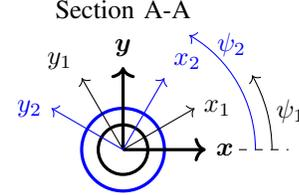
Fig. 2: Each tube has a material-attached frame which propagates along the arc length  $s$  of the robot with its  $z$ -axis tangent to the backbone of the robot. The absolute rotational angle  $\psi_i$  of tube  $i$  is measured with respect to a zero-torsion Bishop frame and changes in arc length if the tube is in torsion.
