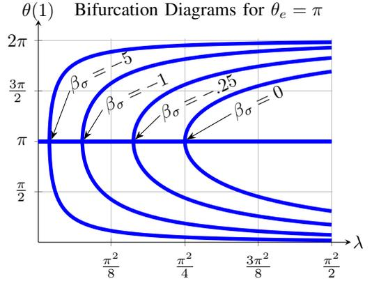
Fig. 6: Bifurcation diagrams are shown for various transmission lengths. As the transmission length grows, the critical bifurcation parameter is reduced.
