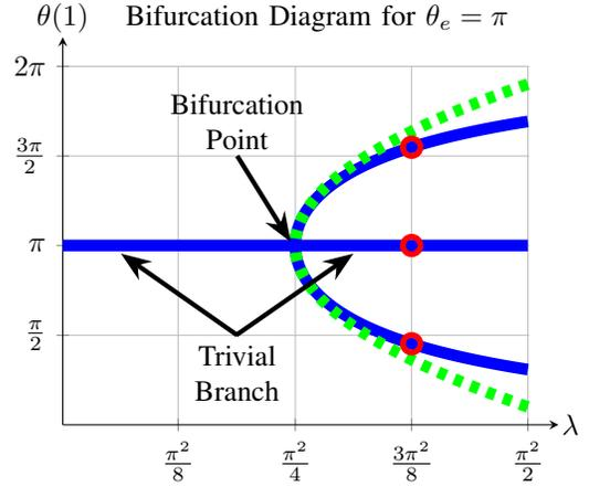
Fig. 4: The bifurcation diagram shows nontrivial branches originating at the bifurcation point  $\lambda = \pi^2/4$  when  $\beta = 0$ . The circles show corresponding points between the bifurcation diagram and the S-Curve in Fig. 3. The green dotted line shows the bifurcation equation solution from (6).
