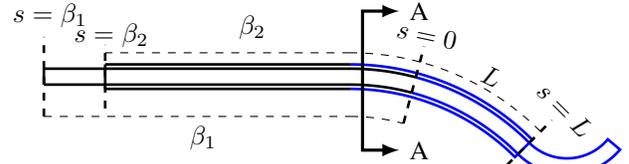
Fig. 1: This diagram illustrates arc length parameter definitions. The blue lines indicate a precurved portion of the tube. We define  $s = 0$  as the most proximal point where the precurved sections of both tubes interact. Note that  $\beta_1, \beta_2 \leq 0$ .
