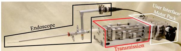
**Fig. 1** This system is made up of three sections: a rigid endoscope that the manipulators pass through, a transmission where rotation and translation are applied to tube bases, and a user interface enabling the surgeon to control the endoscope and both manipulators. See [2] for a detailed description of this robot.
