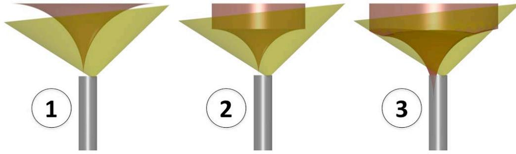
**Fig. 3** Manipulator workspace (red) overlaid on visualization volume (yellow) for: (1) tube design ( $\kappa = 30.1 \text{ m}^{-1}$ , coverage=8.9%) in [2], (2) optimal design ( $\kappa = 47.8 \text{ m}^{-1}$ , coverage=29.5%) with workspace beginning at endoscope tip, and (3) optimal design ( $\kappa = 34.6 \text{ m}^{-1}$ , coverage=64.9%) when the workspace begins a short distance inside the endoscope.
