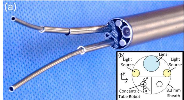
**Fig. 2** (a) Two concentric tube manipulators are deployed through the 8.3 mm endoscope. One aims the laser fiber, and the other retracts tissue. (b) A cross section of the endoscope.
