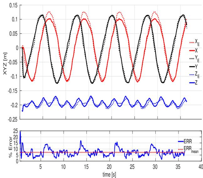
**FIGURE 8:** Dynamic result comparison for phase shifted sinusoidal response with normalized tip error. The dashed lines denote the experimental results while the solid lines represent the simulation results.
