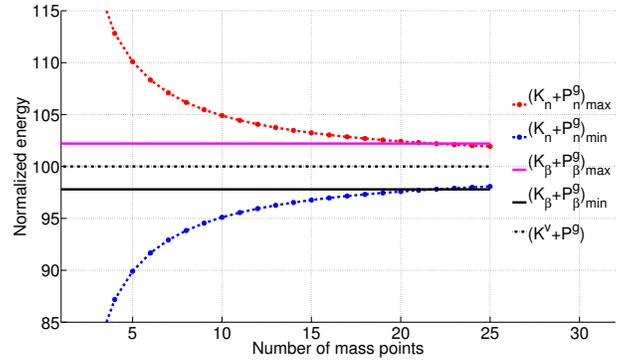
**FIGURE 6:** Normalized combined gravitational PE and KE ranges of  $\mathcal{K}_n + \mathcal{P}_n^g/\mathcal{K} + \mathcal{P}^g$  for different discrete points masses and CoG lumped mass,  $\mathcal{K}_\beta + \mathcal{P}_\beta^g/\mathcal{K} + \mathcal{P}^g$ .
