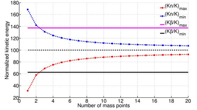
**FIGURE 4:** Normalized kinetic energy ranges of  $\mathcal{K}_n/\mathcal{K}$  for different discrete points masses and CoG lumped mass,  $\mathcal{K}_\beta/\mathcal{K}$ .
