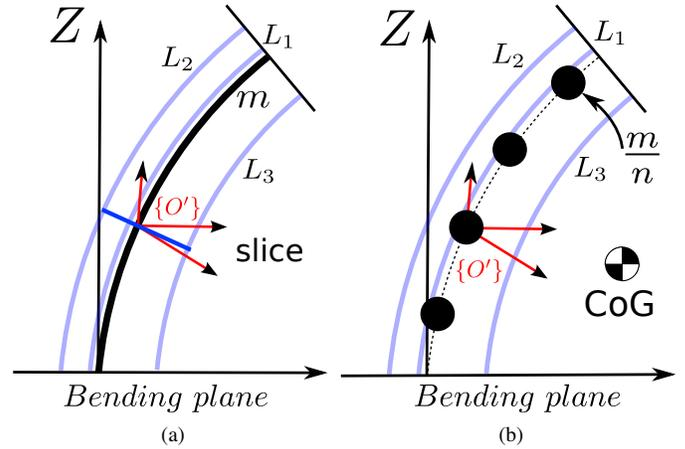
**FIGURE 3:** (a) Schematic diagram of a continuum section with uniformly distributed mass along the length. An infinitesimally thin slice at  $\{O'\}$  is also shown. (b) schematic of a lumped mass system with  $n$  number of point masses along the length. The center of gravity (CoG) is also marked.
