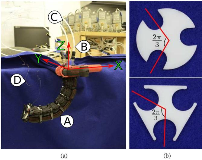
**FIGURE 2:** (a) The pneumatic muscle actuated variable length continuum section: A:-continuum section, B:-pressure supplying tubes, C:-PneuMax 171E2N.T.D.0009S digital pressure controllers, D:-NDI magnetic coil sensor for tip trajectory tracking, (b) rigid PMA mount frame (top right) where the grooves house union tube connectors. The constrainer plates (bottom right) and the grooves support PMA's along the length.
