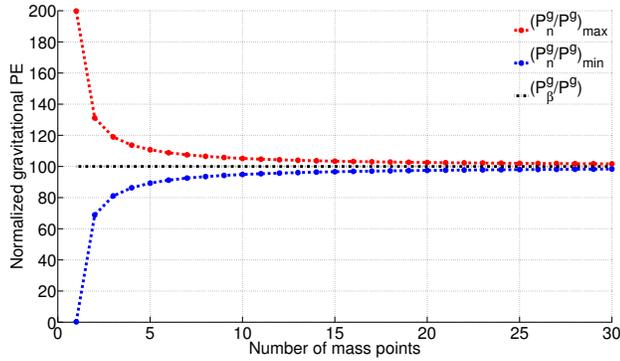
**FIGURE 5:** Normalized gravitational potential energy ranges of  $\mathcal{P}_n^g/\mathcal{P}^g$  for different discrete points masses and CoG lumped mass,  $\mathcal{P}_\beta^g/\mathcal{P}^g$ .
