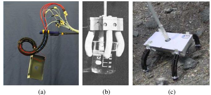
**FIGURE 1:** (a) Serial multisection continuum arm handling an object, (b) continuum sections as gentle fingers of a grasping manipulator (from [10]), (c) continuum sections as compliant limbs of a quadruped robot (from [11])
