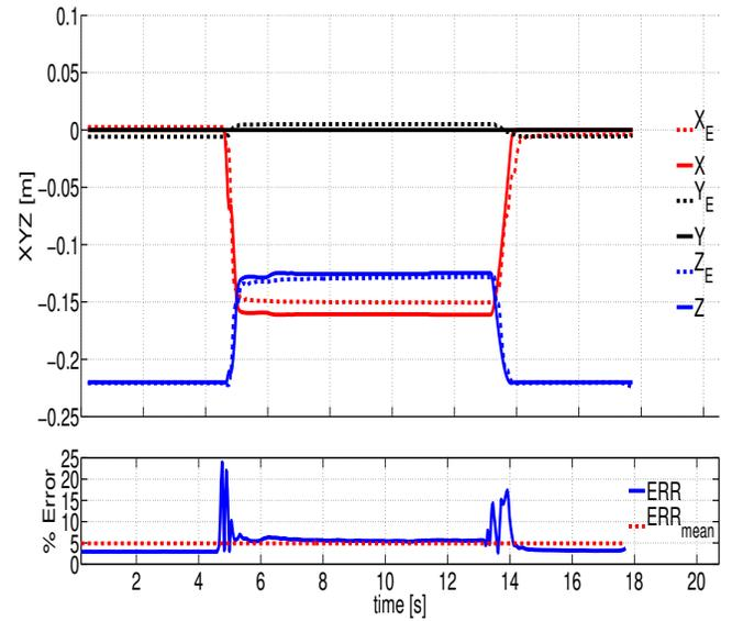
**FIGURE 7:** Dynamic result comparison for rectangular pulse response with normalized tip error. The dashed lines denote the experimental results while the solid lines represent the simulation results.
