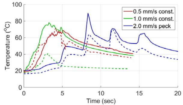
Fig. 4 Mean temperature on plane at a distance of 0.5 mm (average distance of facial nerve) from edge of drill path at middle ear throughout the drilling procedure. The solid and dashed lines represent the first and second trial for the parameter set, respectively.
