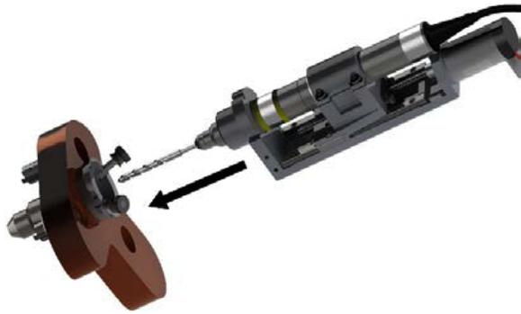
Fig. 2 The automatic drill guide mounts to the microtable and is programmed to drill from lateral skull surface to the cochlea
