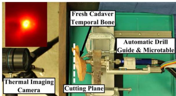
Fig. 3 Experimental setup for evaluating the temperature rise near the facial nerve during minimally invasive CI surgery, and image of heat distribution as the drill enters the middle ear for one trial
