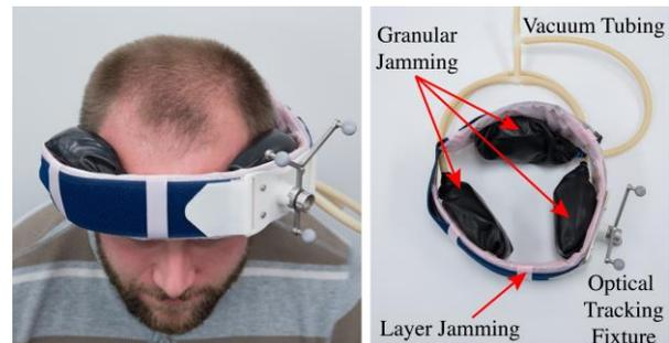
**Fig. 2** Our new fixation device features three granular jamming pads, which conform to the patient’s skull, and are mounted to a layer jamming band that can solidify to hold them in place relative to one another when a vacuum is drawn.
