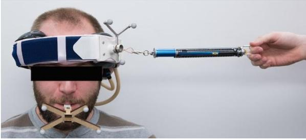
**Fig. 3** The test setup for our experiments applying perturbations to the granular/layer jamming headband. A spring scale was used to pull on the headband in four different directions. The movement of the headband markers with respect to bite block markers was measured using an optical tracker as force was applied by hand using the spring scale.
