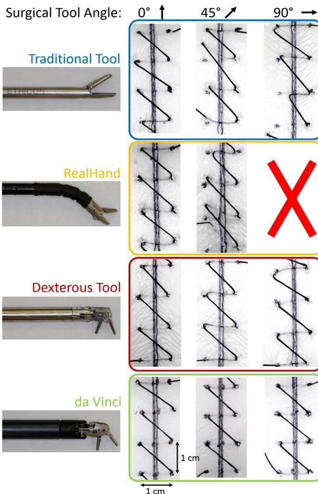
Fig. 10. Results of suturing experiment at three tool angles for, from top to bottom, the traditional laparoscopic tool, the RealHand, the dexterous tool, and the da Vinci robot. The subject was unable to complete the  $90^\circ$  suture with the RealHand.
