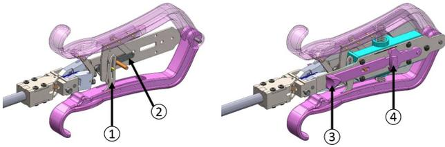
Fig. 8. Dexterous tool handle, showing ① grasp locking mechanism, ② Z-bar mechanism, ③ lock release button, and ④ lock disable switch.
