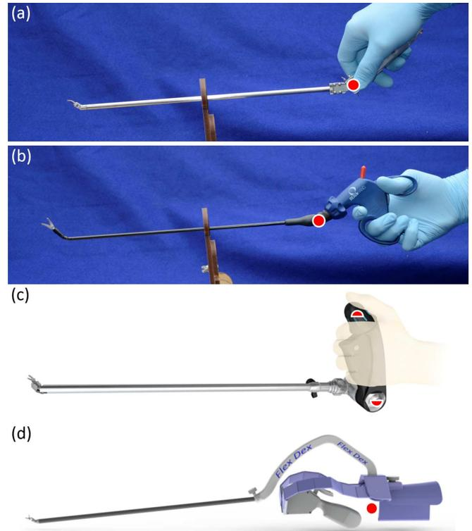
Fig. 2. A comparison of control point location for (a) the new tool described in this letter, (b) the RealHand, (c) the Radius, and (d) the FlexDex instrument. The new tool is the only one that places the control point within the user's grasp as the da Vinci robot's user interface does.
