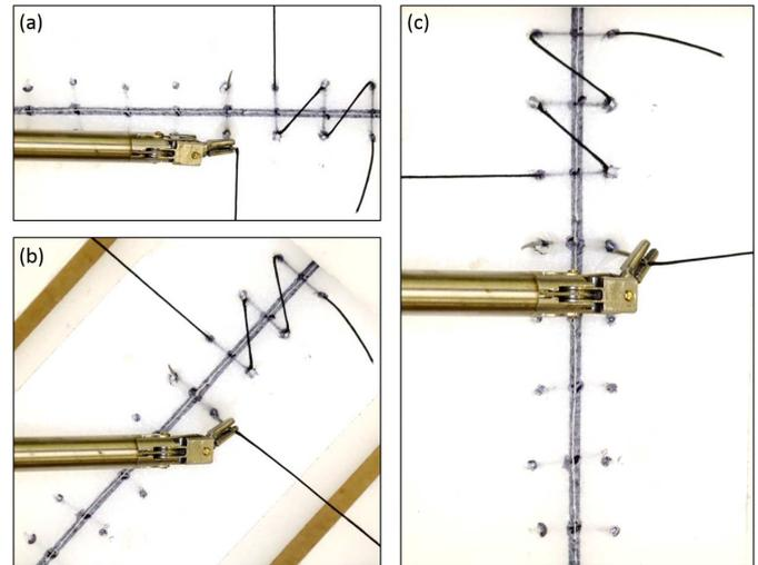
Fig. 9. Surgical tool angles for suturing experiment, showing the dexterous tool throwing sutures at ① 0°, ② 45°, and ③ 90° angles.
