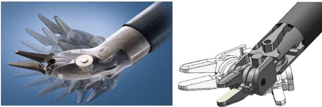
Fig. 5. The distal wrist (right) provides articulation similar the da Vinci EndoWrist (left) [20]. Cables are not shown; routing is illustrated in Fig. 6.
