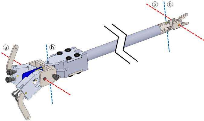
Fig. 4. Control point mapping: axes of rotation in the proximal wrist joint (left) are mapped to the distal wrist joint (right).
