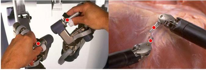
Fig. 1. The da Vinci robot user interface maps motion of control points located between the user's fingers to corresponding control points on the instruments inside the patient. Image source: <http://www.intuitivesurgical.com/>, control point illustrations added.
