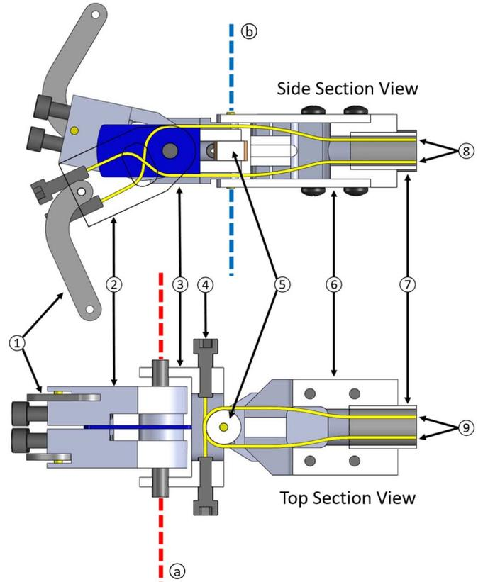
Fig. 7. Side and section views of handle mechanism, showing ① linkage connecting pulley arms to handle, ② pulley arms, ③ proximal wrist, ④ vent screw, ⑤ center pulley, ⑥ cable guide, ⑦ rod, ⑧ cables for one gripper of end effector, ⑨ cables for end effector lateral wrist pulley, and control axes.
