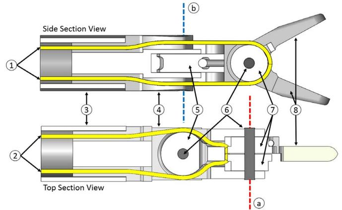
Fig. 6. Side and top section views of the distal wrist mechanism, showing ① one set of end effector gripper cables, ② lateral wrist cables, ③ rod, ④ cable guide, ⑤ lateral wrist pulley, ⑥ pins, ⑦ end effector gripper pulleys, ⑧ end effector grippers, and control axes. Cable management is addressed via the grooves shown in Fig. 5 (right).
