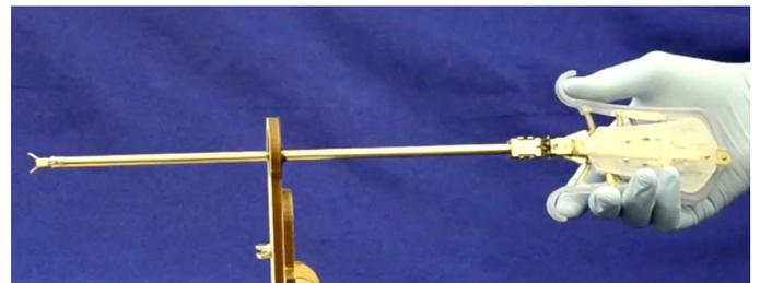
Fig. 3. The dexterous tool, showing distal wrist (left), proximal wrist (right), and handle. The control point (see Fig. 2 for control point illustration) is between the thumb and forefinger, and the end effector grippers are closed by squeezing the handle.
