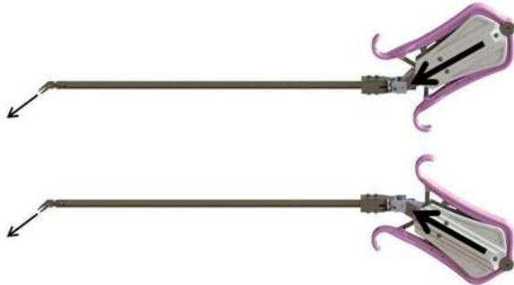
**Figure 4.** Kinematic mappings for laparoscopic tools with wrists: parallel (top) and reverse (bottom). The instrument used in this example is the Vanderbilt Maestro.
