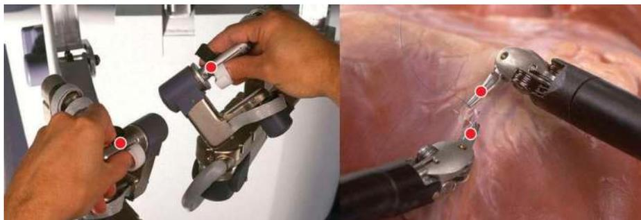
**Figure 15.** Demonstration of control point concept in robotic master-slave: the da Vinci robot user interface maps motion of control points located between the user's fingers to corresponding control points on the instruments inside the patient. Image source: [59], © 2016 Intuitive Surgical, Inc., control point illustrations added.
