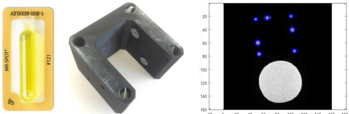
Fig. 1: Previous Z-marker concept of [1] including seven of the Gd-based marker capsules (left) that are inserted into the 3D-printed frame (middle). This marker concept provides a distinct resonance pattern in the MR-image with a fiducial registration error of  $FRE = 2.10$  mm (seven white dots, right)[1].
