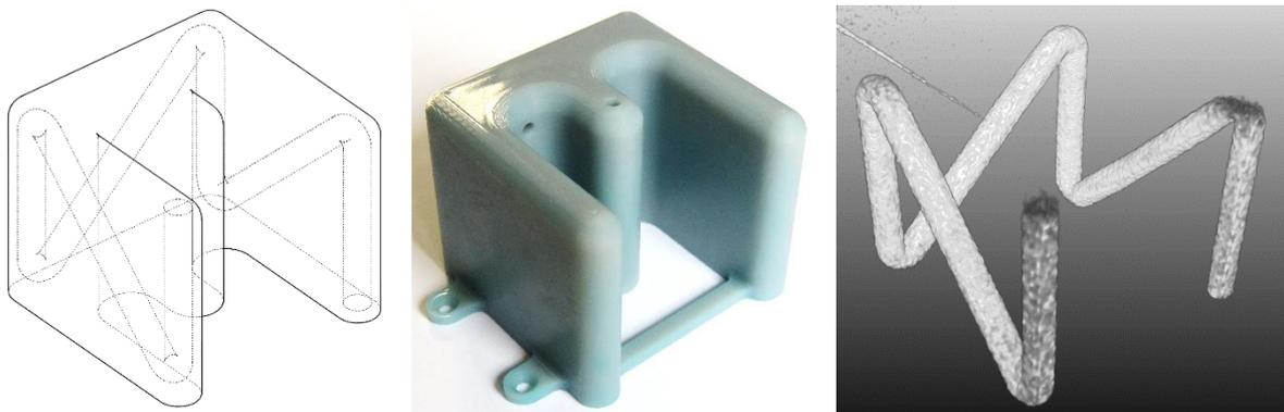
Fig. 2: The Z-RP-MR-marker with the distinct shaped internal tunnels in the CAD-view (left), the printed marker without any openings to the outside (middle), and the measured 3D-MR-image of the Z-shaped tunnels (right, 0.5 mm per voxel).
