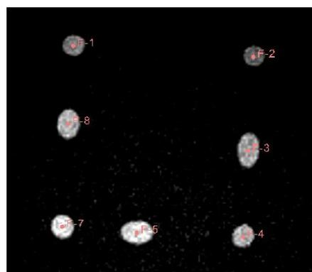
Fig. 3: View of a single MR-image plane (0.5 mm per voxel) showing the seven tunnels in cross section which are used as marker points to determine the instrument alignment.
