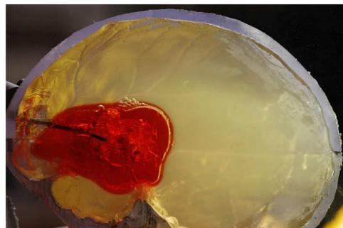
Fig. 7. Phantom gelatin model of an intracerebral hemorrhage (red) within a plastic skull and a steerable cannula for blood evacuation.
