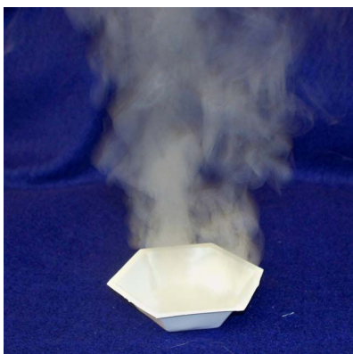
Fig. 4. A large amount of Oxygen was produced when a small amount of liquid Hydrogen Peroxide was catalyzed by a silver screen.
