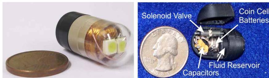
**Fig. 12** (Left) Prototype capsule developed by Lenaerts *et al.* (©2007 Elsevier) [102], which is capable of transmitting 150 mW through inductive coupling. (Right) The prototype fluid-powered capsule of Toennies and Webster [88]
